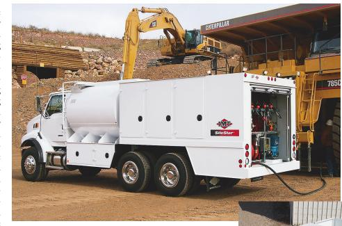
This new SiteStar lube truck incorporates an elliptical fuel tank positioned ahead of the redesigned body, which features three added street-side storage compartments.
