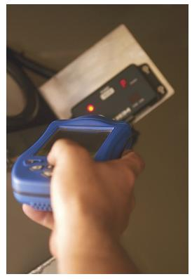
Upon completion of the refueling, the fueler scans the Pump Tracker module, which confirms how much fuel was put into the machine. This data becomes part of the record for each individual machine, helping S.W. Rodgers build its maintenance history.
