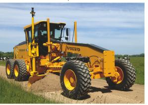
duced G900 Series motor graders. The operators used two G940s, one with a conventional 8-speed transmission, the other with the new 11-speed, to grade a county road, to trim roadbase limestone, and to hog out dirt in a ditching exercise.
