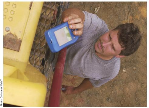
Fueler Doug Caldwell scans a machine before fueling. Data such as model number and hours are collected. The system then indicates how much fuel the machine is supposed to receive.
