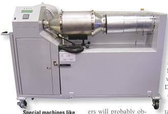
Special machines like this will clean diesel particulate filters with compressed air. Most dealers will have them, and will also offer clean filters on an exchange basis. Caterpillar DPFs can be cleaned while still on trucks.
