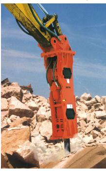
According to NPK, all of its breakers are built with only two moving parts, are designed to eliminate bladdertype accumulators, use a quickchange tool system and feature separate ports to accommodate an Auto Lube system and an air line for underwater operation. The company's medium and large models use a shock-absorbing mounting bracket with heavy-duty rubber pads to ab-
