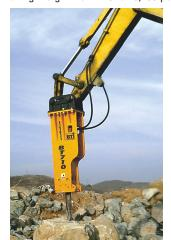
includes a mix of side-plate models (TB-ME, TB-QA and TB-X) and boxed-housing models (TB-XC and BT-Series) that accommodate a wide spread of carriers, including pedestals.
