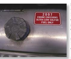
New engines need ultra low-sulfur fuel, so current higher-sulfur fuel should not be put in the new trucks' tanks.
