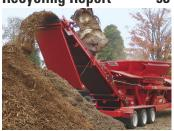
Tub grinder built with purpose
