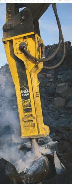
Technical advances in today's mounted hydraulic breakers include, for example, the ability to tailor start-up/shut-down behavior and to adjust the impact energy/ blow-frequency ratio to suit the operating situation. Also, more breakers today are running with automatic greasing systems, they're quieter than ever before, and they are being engineered for protection against on-site hazards, including inexperienced operators. And lest we forget, they're also easier to service.
