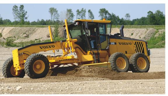
Gord Diamond makes a heavy push during the ditching exercise. Our other guest operator, George McHattie, used the G940's control features to advantage during this exercise: "I didn't once touch the foot throttle or the inching pedal when making turns at the end of the ditch. I planted my feet on the floor and used the panel switch for engine speed and made directional shifts without the inching pedal. Very nice features."
