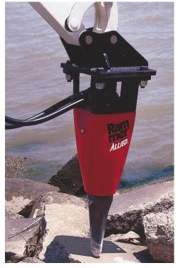
The "unbreakable" tool for Allied's Rammer in-Series is designed to resist binding by virtue of its trapezoidal shape, side-relief contours, and 5-inchdiameter construction.
