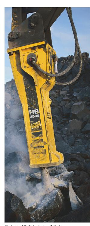
Illustrative of the technology available for today's hydraulic breakers, the Atlas Copco HB 2500's start-up/shut-down behavior can be tailored to the operating situation; it can adjust the impact-energy/blow-frequency ratio; and it uses an automatic greasing system.
