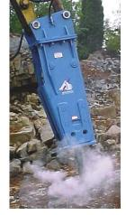
steels that provide long-wear life in severe applications. Large upper and lower tool bushings are designed with special, wear-resistant alloys.
