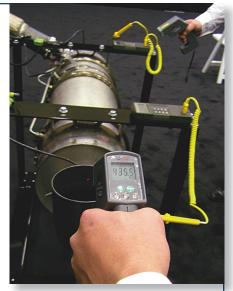
Temperatures at tail pipes could exceed 1,000 degrees F, but measurements show that the heat dissipates fast when the exhaust hits the outside air.
