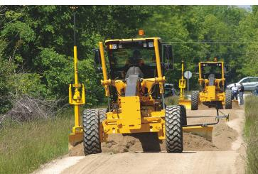
Both operators agreed that when grading this gravel road, the 11-speed provided smoother overall operation, especially when changing gears.
